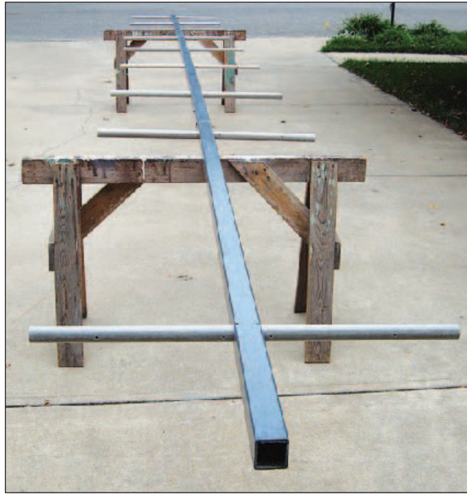
Figure 2 — Assembled boom and splicers.
